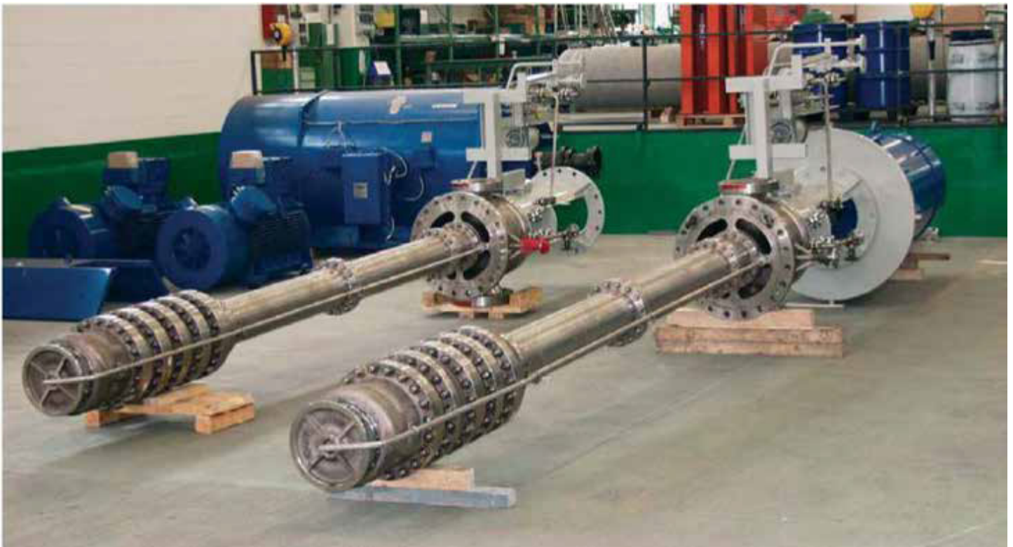
VBN pumps in Gabbioneta test room
